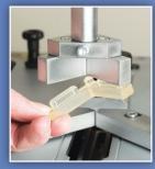
Enables a quick change to a different clamping pad depending on joining applications
